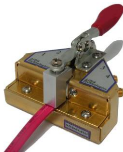
Figure-3:SATA-RW01AM (with DUT)
